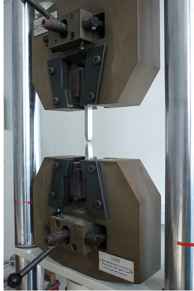
Figure 2: Machine à essai de traction.
